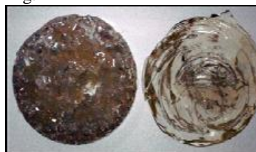
Figure 2. Alginate dispersed in PPF (left) Pure PPF (right)
