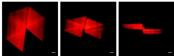
Figure 3. 3D projection of fluorescent-acrylate-PEG-RGDS pattern in PEG-DA.
