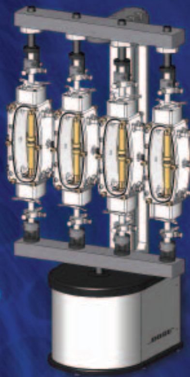
Multi-specimen BioDynamic™ Test Instrument for Compression Loading of Orthopaedic Tissues
