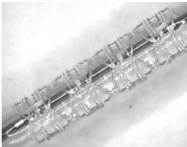
**Figure 1:** A balloon-expandable, slide-and-lock CASPER stent.
